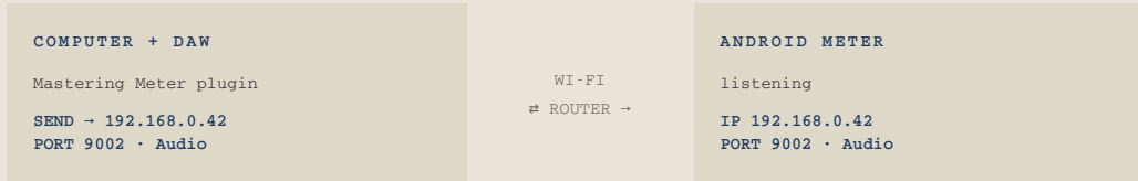
FIG. 4.1 — THE PHONE'S IP IS THE PLUGIN'S DESTINATION. BOTH ENDS USE THE SAME AUDIO PORT.
